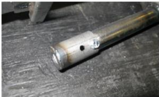
NG Air Collar Installed
